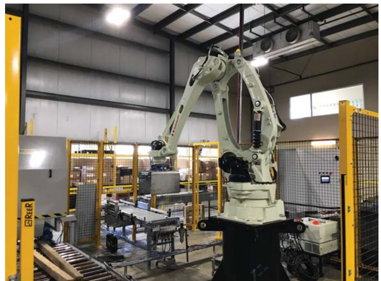
This pedestal-mounted Kawasaki CP180L was able to maintain production speeds while eliminating ergonomic concerns for operators.
