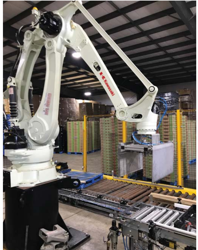
The custom tool designed by Caxton-Mark allows for damage-free loading of product
