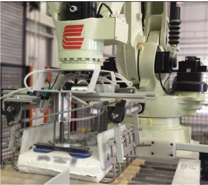
The custom end-of-arm tool, designed by Conveying Industries, securely picks each bag off the conveyor at a rate of 18-20 bags per minute.
