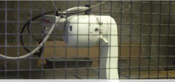
Kawasaki RS080N robot, retrofitted with a paint gun, sprays liquid cement into faux stone molds on conveyor.
