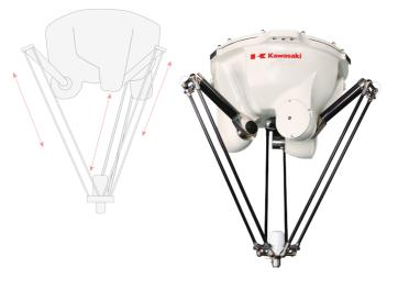
**PARALLEL LINK ROBOT (DELTA)** When speed is key
