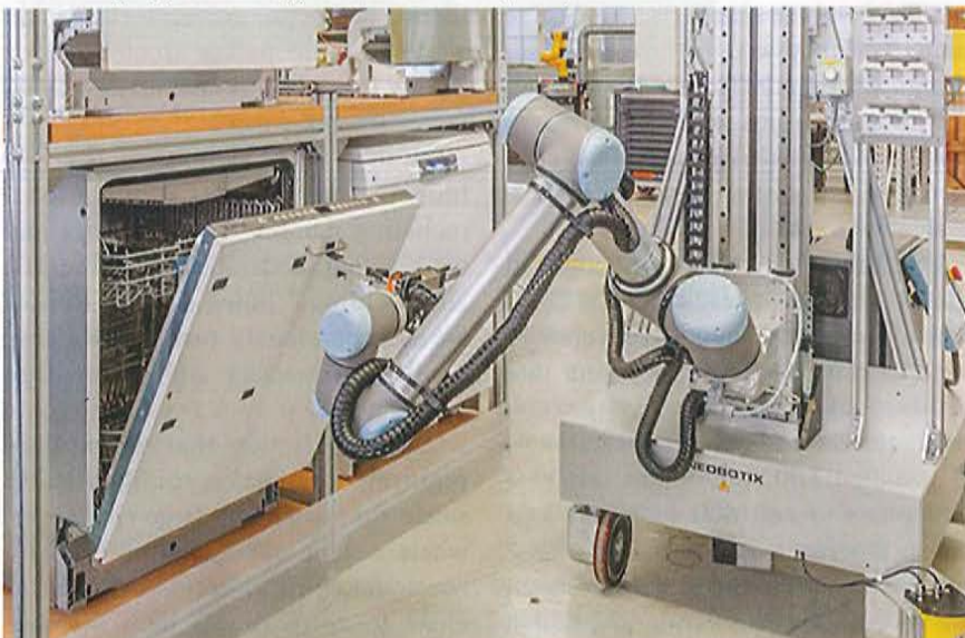
Engineers at BSH Hausgerate GmbH use robots to test dishwashers. They also use robots to apply silicone liners inside refrigerator doors. Photo courtesy Sick AG
