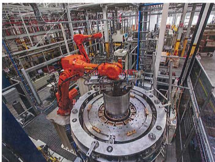
Six-axis robots are used to assemble washing machine parts. Photo courtesy Gorenje Group
