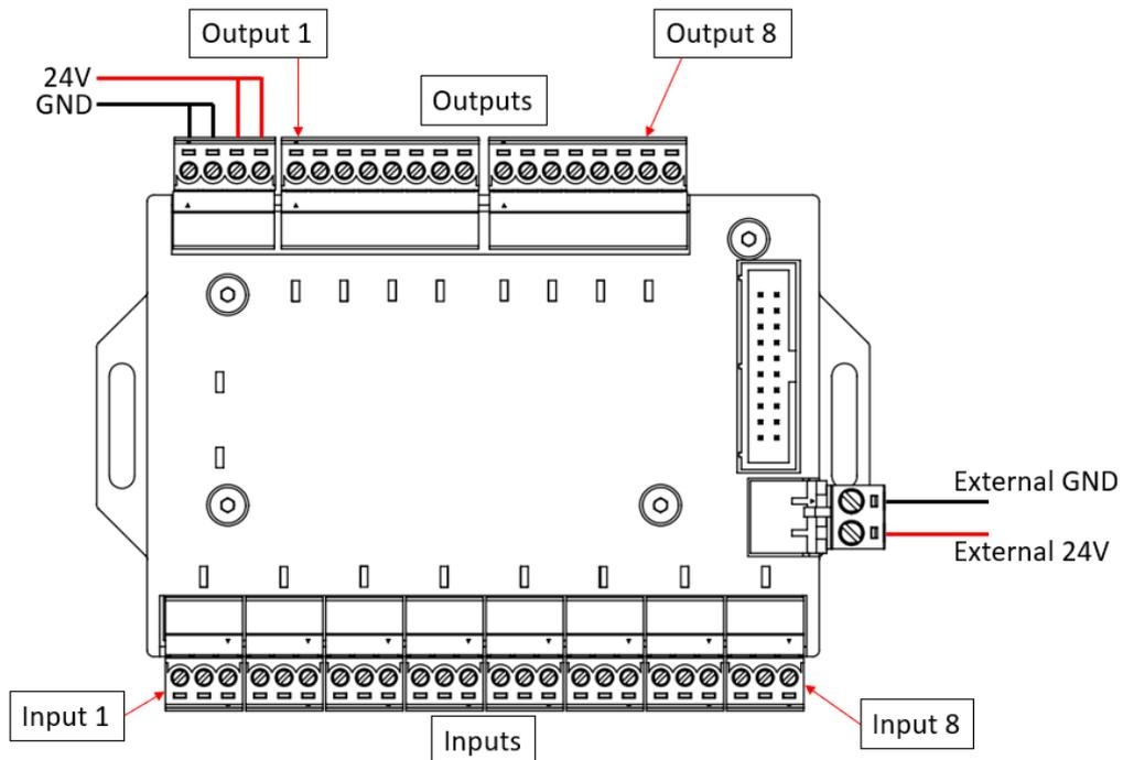
A total of 8 24V inputs and 8 24V outputs can be connected.
