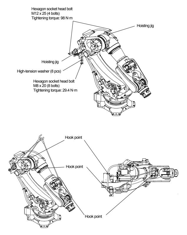
Hexagon socket head bolt M12 x 35 (2 bolts) Tightening torque: 98 N·m Hexagon socket head bolt M12 x 45 (2 bolts) Tightening torque: 98 N·m Hoisting jig High-tension washer (2 pcs) Hexagon socket head bolt M12 x 35 (2 bolts) Tightening torque: 98 N·m Hook point Hook point Hook point
