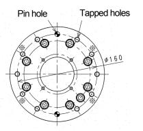
In the robot arm end section, a flange is provided on which hand, gun, or other tools are mounted. Screw the mounting bolts into the tapped holes on the circumference of  $\phi$ 160 on the flange, referring to the figure on the left. Moreover, position the tool by utilizing the pin holes.
