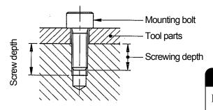
Select mounting bolts with proper length to secure the specified screwing depth according to the tapped depth of tool mounting flange. Use high tension mounting bolt and tighten them to the specified torque.
