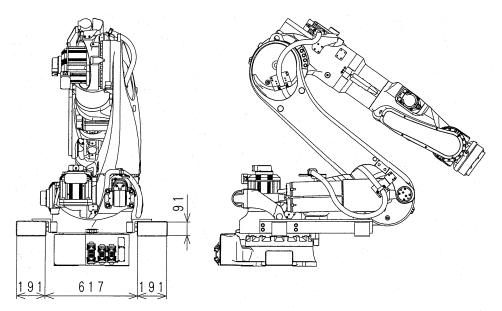
Attach the transportation jig as shown in the figure below.
