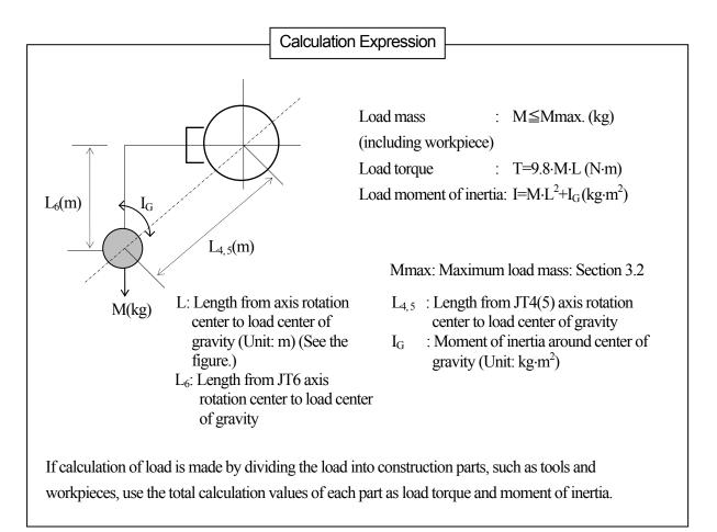
Regarding the load on the robot wrist section, meet the following restriction conditions:
