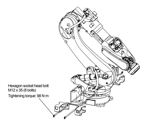
The hoisting jig shown above can be used to hoist up BX200X, BX250L, and BX300L. For the hoisted up postures, refer to the table in section "4.1.2 Fastening Wire Sling Directly on The Arm."
