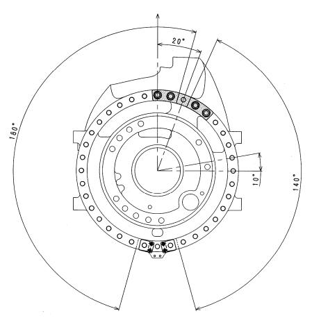
For BX200X, BX250L and BX300L, the motion range is 180° on both plus and minus sides due to the restriction from control and harness treatment and total motion range of both plus and minus sides is 360°. Do not change the mounting position when mounting a stopper block because the motion range on plus (or minus) side exceeds 180° if the mounting position is changed.
