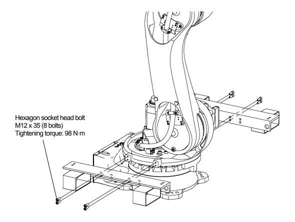
B Series Kawasaki Robot Installation and Connection Manual
