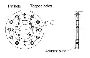
When passing a cable/hose through the wrist hollow section, clamp is attached on the wrist flange as shown in the left figure. Provide a hole of  $\phi$ 100 on the flange of the tool side, or use an optional adapter plate or an adaptor bracket (option, standard for BX250L/300L).
