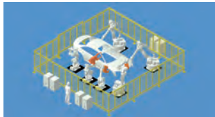
Simultaneous simulation of multiple robots is possible.
