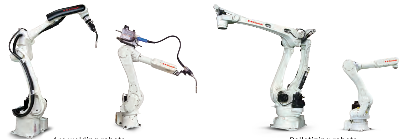
Arc welding robots
