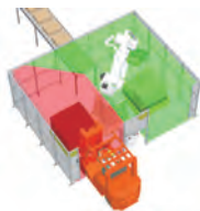
Limiting the motion range according to operator's working area.
