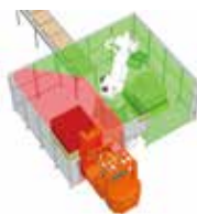
Limiting the motion range according to operator's working area.
