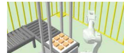
Compensation of the gripping position by fixed or hand cameras.
