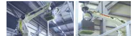
There is no need to register varieties and stacking patterns in advance, and it can handle unknown workpieces and random placements.
