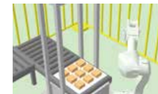
Compensation of the gripping position by fixed or hand cameras.
