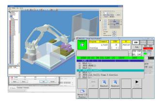
Load data to robot, and touch up key pick & place positions
