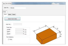
Define pallet and workpieces parameters
