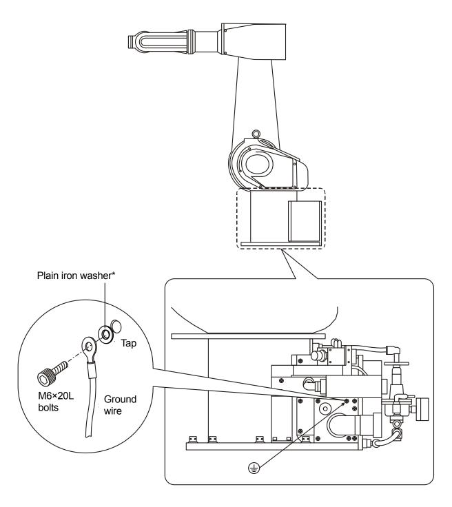
\* Insert a plain iron washer between the arm and the ground wire to secure ground and to avoid corrosion.
