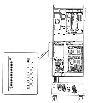
Brake release switch position
