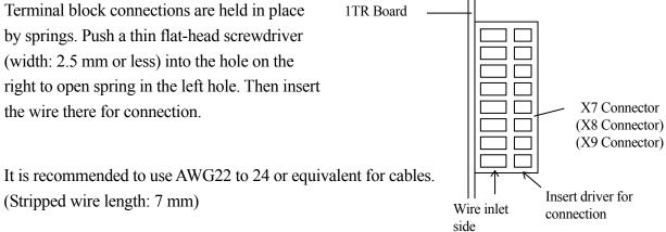
To assure the wiring, we recommend using ferrules;
