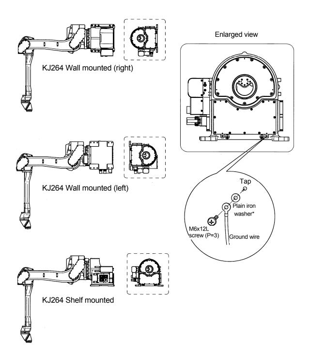
\* Insert a plain iron washer between the arm and the ground wire to secure ground and to avoid corrosion. The above figure shows KJ264 as an example. The connecting point of ground wire shown above is the same as that of KJ194 and KJ244.
