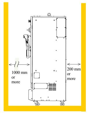
3. The inlet port for air-cooling is on the rear upside of the controller, and the air exhaust port is on the rear downside.
