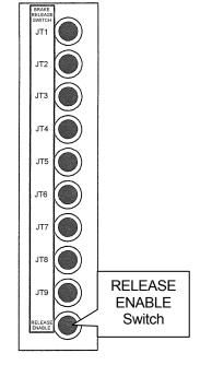
Robot brake release axes
