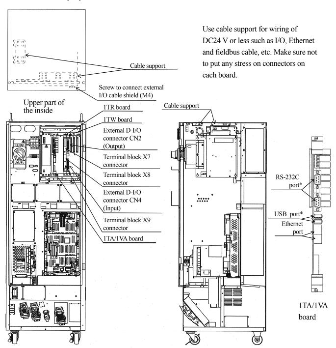
See the upper right figure for details on connecting ports of 1TA/1VA board.
