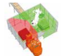
Limiting the motion range according to operator's working area.
