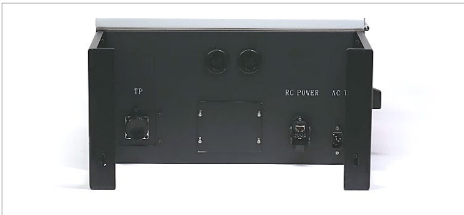
Fig. 44: Connections of Controlbox (bottom view)
