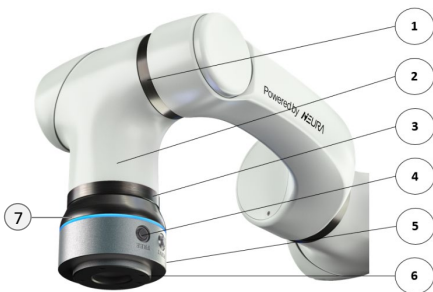
Fig. 3: Overview axis module 5/6 and TCP (CL1)
