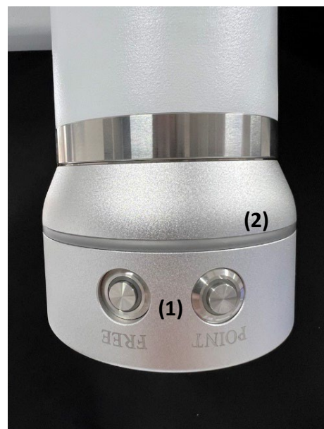
Fig. 42: Robot TCP flange with TCP (HMI) buttons
