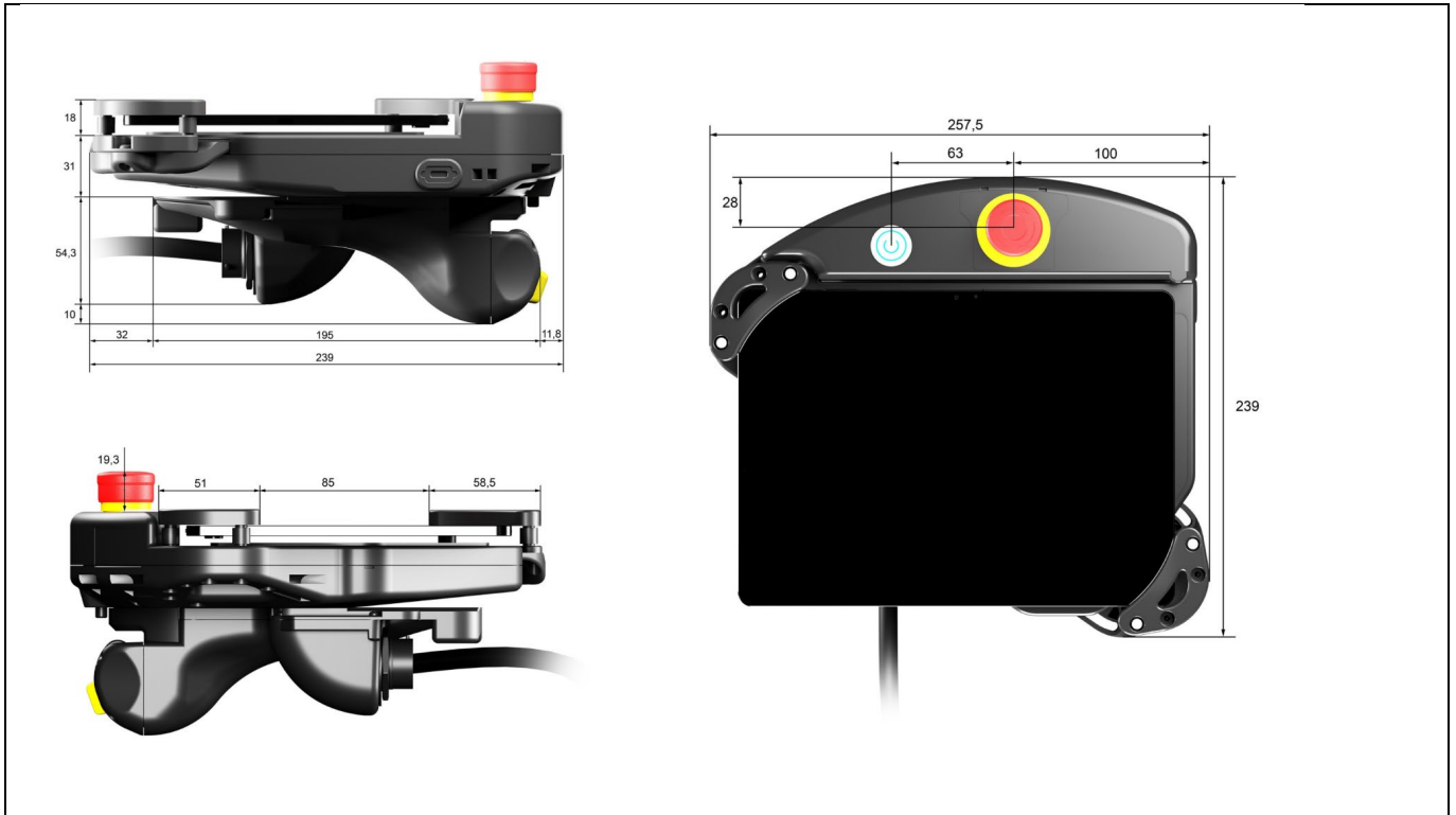
Fig. 12: Size and dimensions in mm - Teach Pendant
