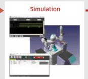
The movement of robots and peripheral devices, as well as interference conditions when models come into contact, can be displayed, allowing you to prevent system problems before they occur. You can also check the status of currently executing program steps and signals, shortening the time it takes to find problems.
