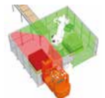
Limiting the motion range according to operator's working area.
