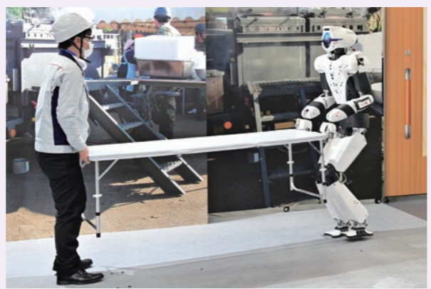
Kaleido, a humanoid robot, working with a human partner to lift and move heavy objects
