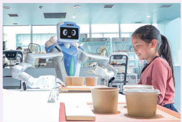
Nyokkey, a self-propelled robot with arms serving at a restaurant open to the public as part of demonstration testing
